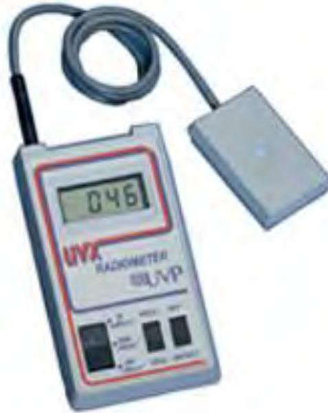
This digital UVX Radiometer is used with one of the three interchangeable sensors (ordered separately) for measuring 254nm, 365nm and 302nm UV wavelengths.
