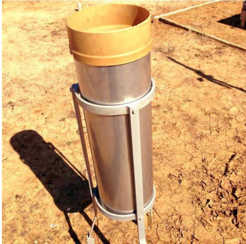
An instrument used to measure liquid precipitation by meteorologist or hydrologists; often the amounts used to estimate crop yield.
