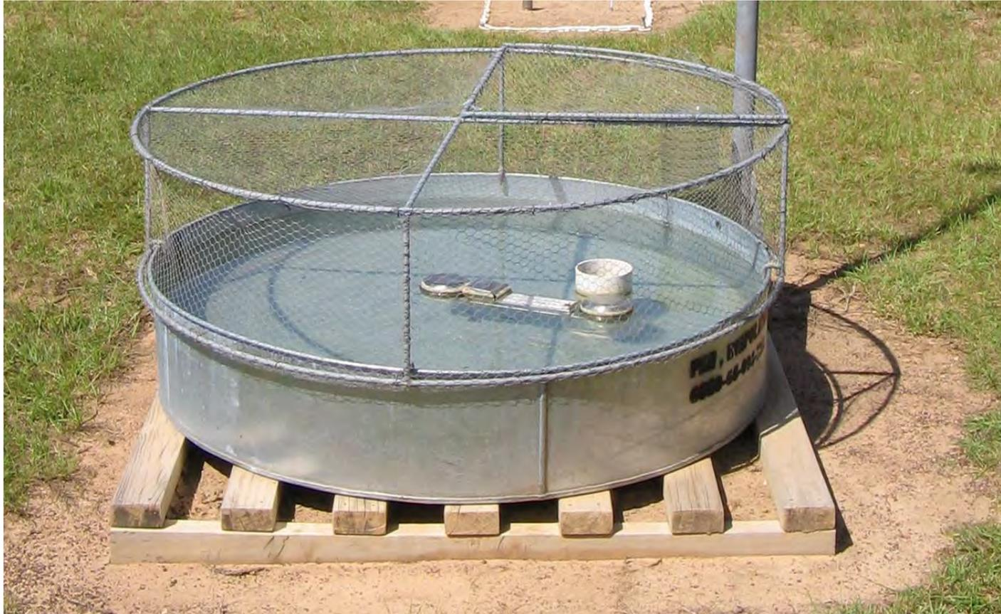
A cylinder or circular pan with 120.7 cm diameter, 25 cm in height is used to measure evapotranspiration; this provide guidance for irrigation of the crops.
