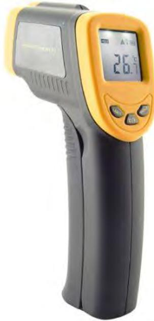
An infrared (IR) thermometer measures the thermal temperature of the plant leaves or a crop canopy. Once plants go into water stress, they begin to close their stomata and cease to transpire, causing the plant to "heat up" and the canopy temperature to rise.
