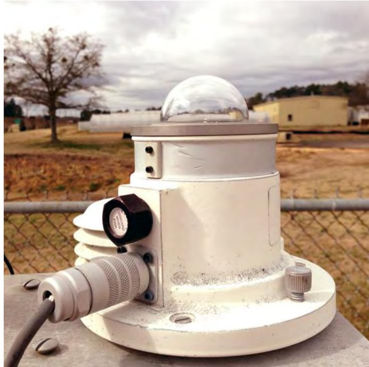
This gadget measures Sun's UV-B radiation from 280-320 nm; measured UV radiation is being used to project Harmful Sun's UV so that beach goers can apply the right kind of sunscreen lotions (SPF) to protect against cancer causing radiation.
