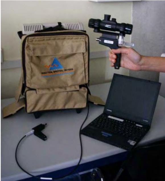
The FieldSpec portable spectroradiometer offers the modular Goetz spectrometer engine with a spectral range from 350 nm to 2500 nm
