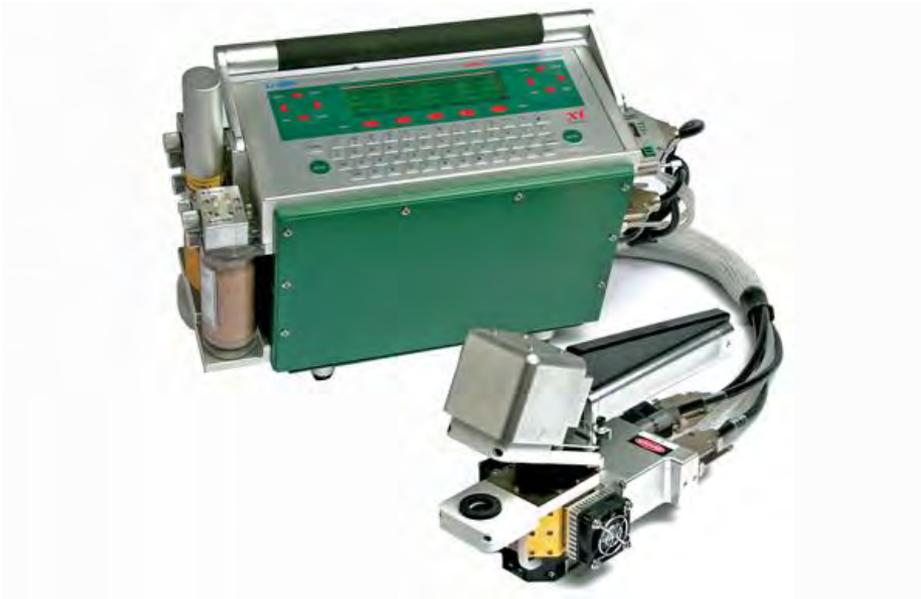
The LI-COR 6400 utilizes gas exchange principles to measure the photosynthesis rates of plants.
