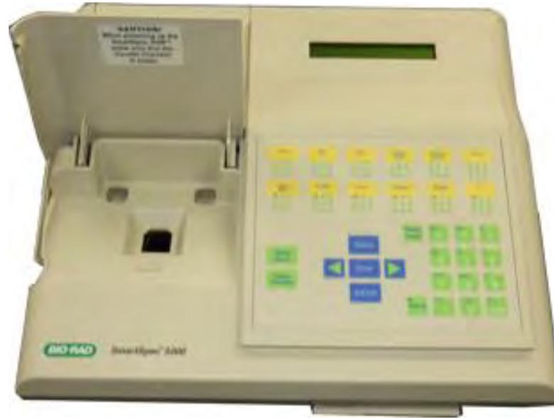
The UV/visible SmartSpec 3000 spectrophotometer has a working wavelength range of 200–800 nm.
