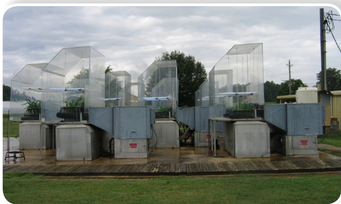
Sunlit growth chambers known as Soil-Plant-Atmosphere-Research (SPAR) units, Mississippi State University, Mississippi State, MS used in the current study.
